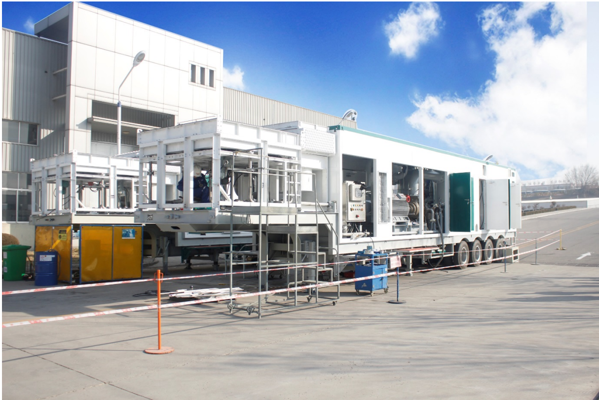
Figure 1: Jerel Truck Mounted Electric-driven Screw Compressor Package on Their way to Russia
