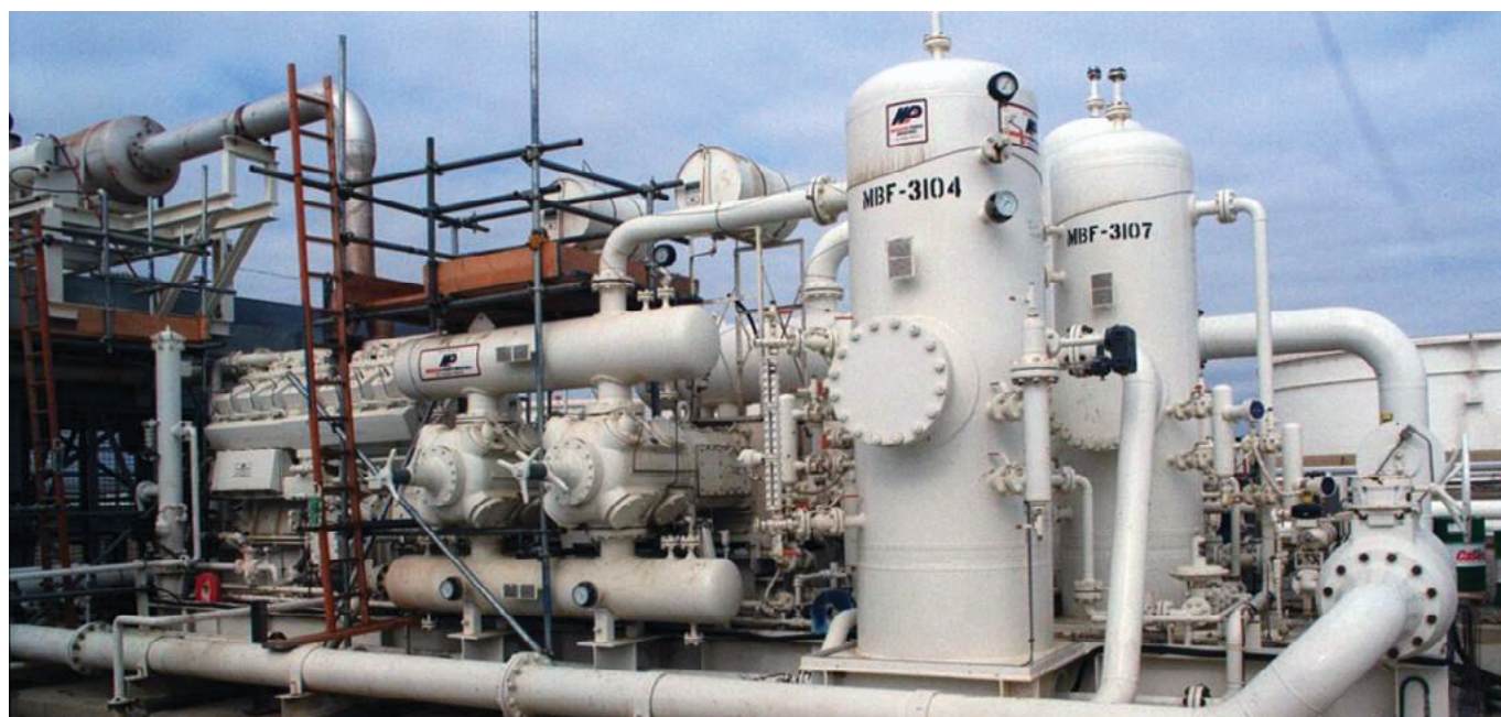
Azerbaijan International Operating Company (AIOC), Baku, Azerbaijan. Compressor packages with Ariel JGD/4 driven by gas engine 890 kW.
