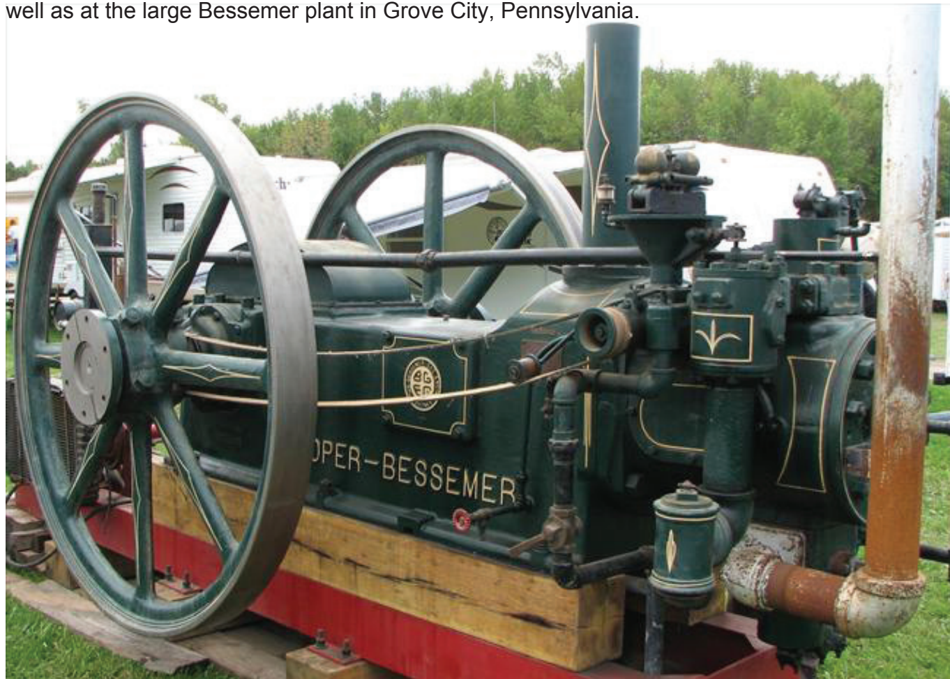
Four-cycle one-cylinder horizontal gas engine had been produced at Mount Vernon from 1930 to 1985.
